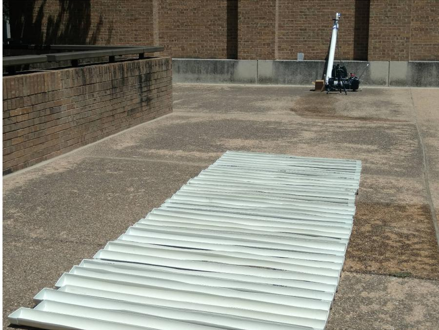
Figure A.2: Troughs for water distribution measurements.
