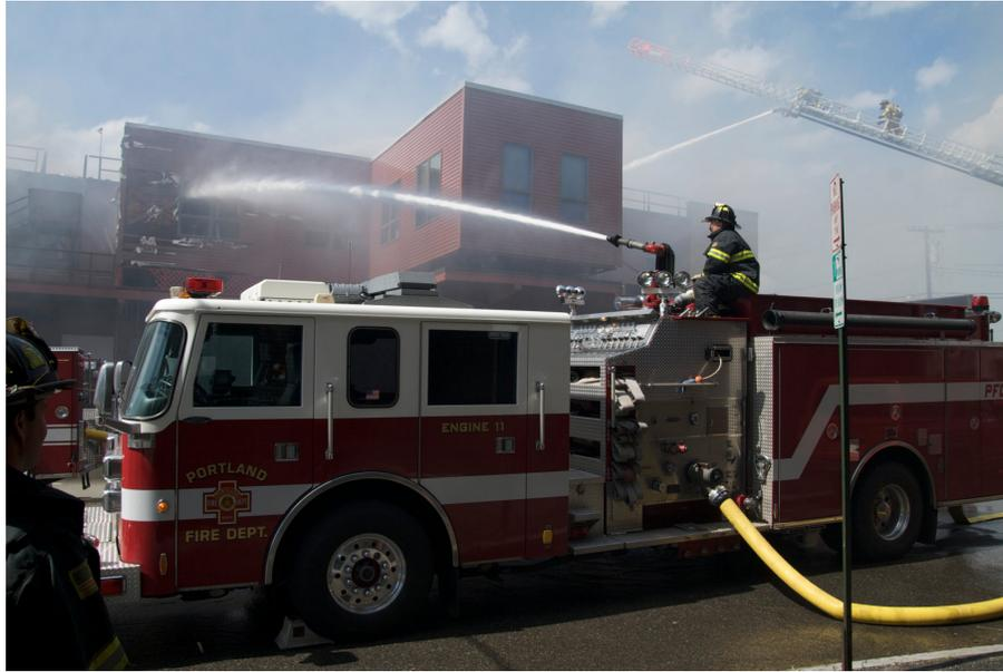
Figure 7.1: Two fire monitors in use by the Portland Fire Department. Fire monitors can deliver 5000 GPM ( $\sim 300$  L/s) or more through nozzles up to and beyond 3 inches ( $\sim 7$  cm) in diameter, leading to maximum ranges of 200 meters or more. Photo from [https://en.wikipedia.org/wiki/File:Deck\\_gun\\_on\\_American\\_fire\\_engine.jpg](https://en.wikipedia.org/wiki/File:Deck_gun_on_American_fire_engine.jpg).
