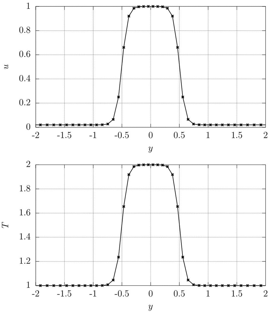
*Figure 3.5:* Inlet profiles for the jet cases in this work. The temperature plot is an example — the maximum temperature is a parameter that was varied in the simulations. Points correspond to actual grid points.
