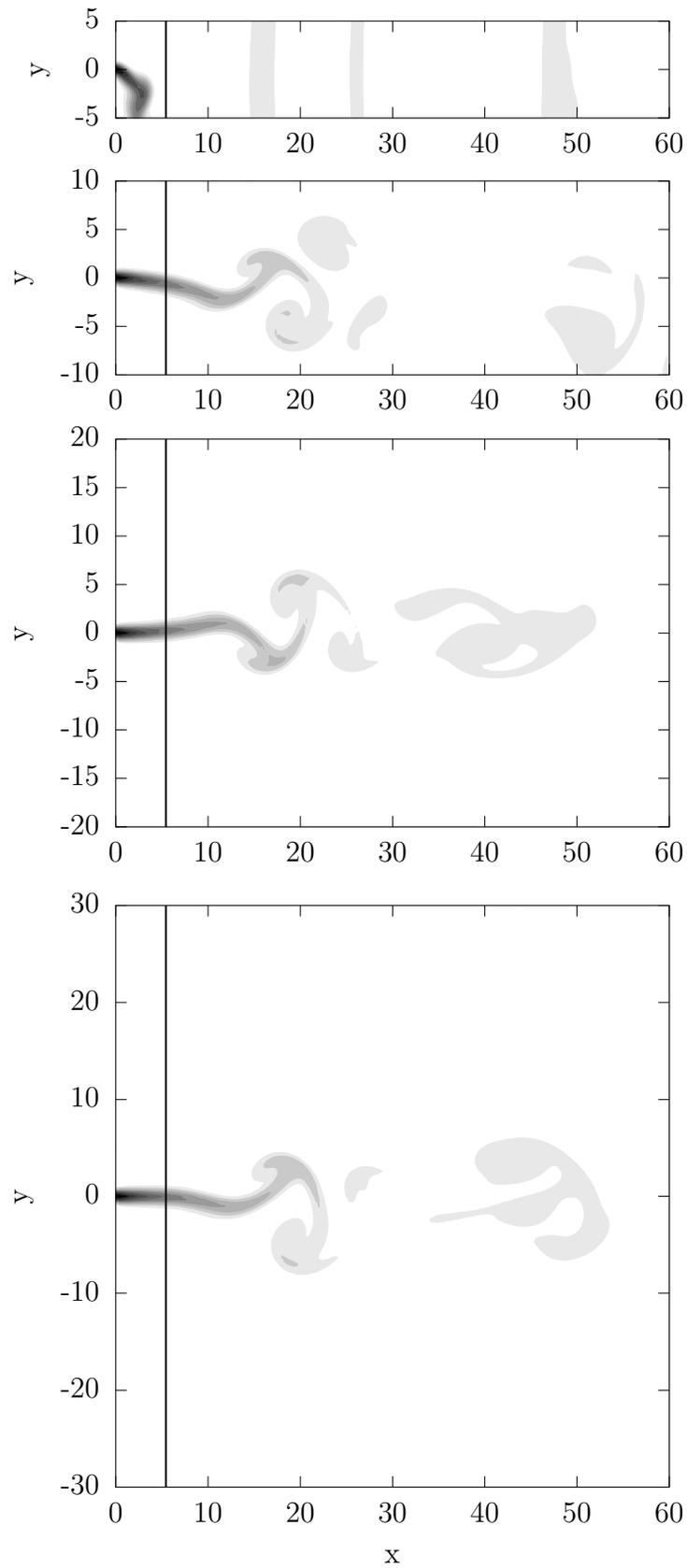
*Figure 3.6:* Temperature contours for cases with different domain widths. Black is  $T = 1.5$ . White is  $T = 1.0$ . The black line is where  $Ra_x = 0.5 \times 10^7$ , which corresponds approximately to where the turbulent transition occurs.
