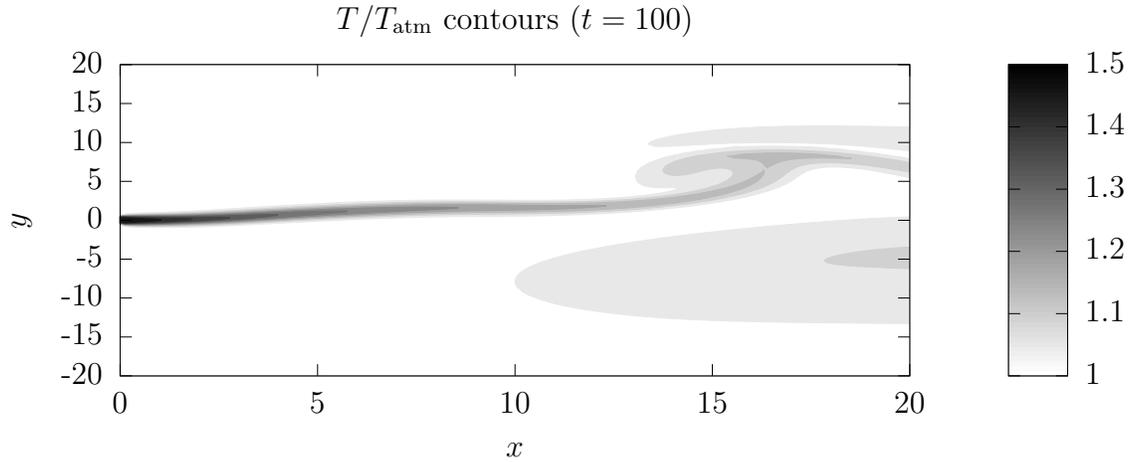
Figure 3.10: Temperature contours for short domain, no sponge-layer case.
