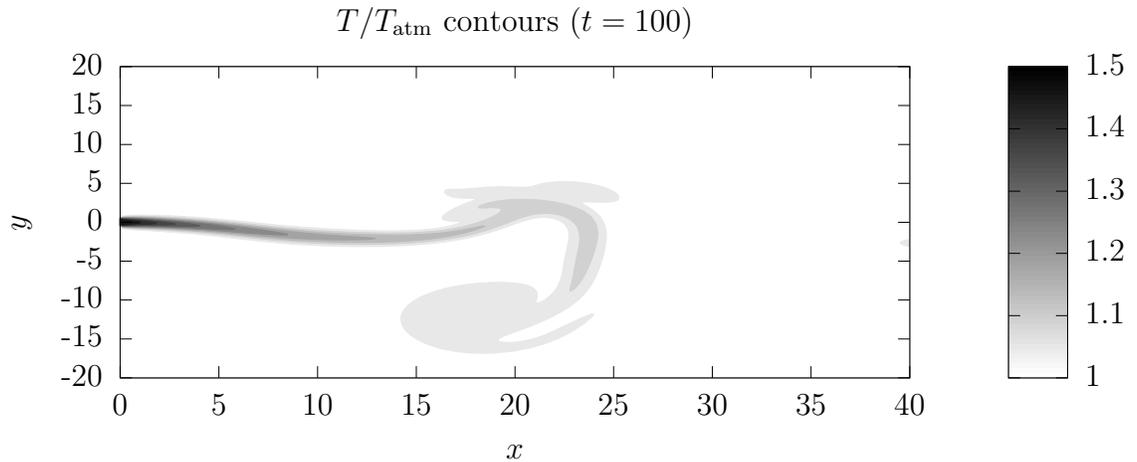
*Figure 3.8:* Temperature contours for long domain, no sponge-layer case.
