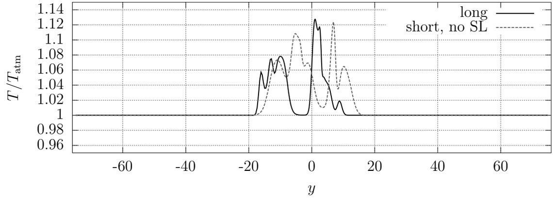
Figure 4.95: Temperature at the outlet for short domain, no sponge-layer case.
