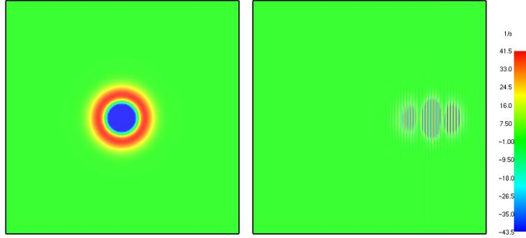
*Figure 1.2:* Unphysical reflection of vorticity off of an open boundary on the right side as seen in FDS [Tre13]. The left figure is the initial condition, which was initialized traveling to the right. The vorticity should be zero everywhere in the right figure.
