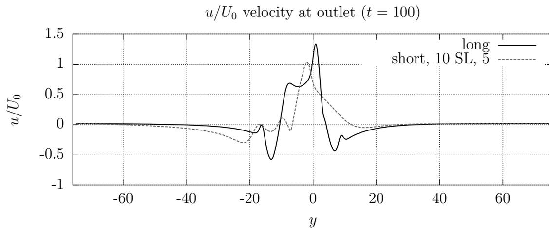
Figure 4.98:  $u$ -velocity at the outlet for short domain, 10 unit sponge-layer with 5-times viscosity increase case.
